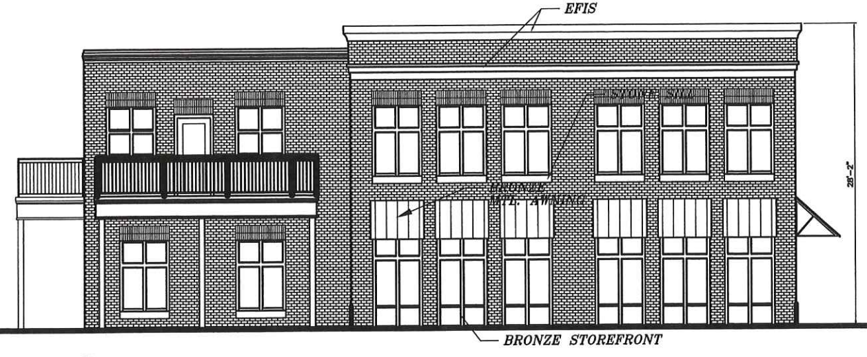
1 A1.0 NORTH ELEVATION SCALE: 3/16"=1'-0"
